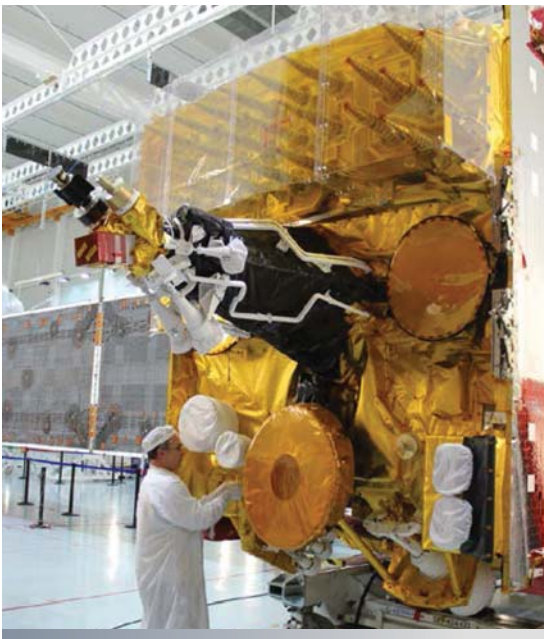
Express AM4R integration in the cleanroom
