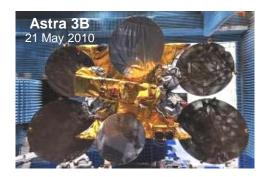
Always enhancing mission capacity: accommodating more antennas, increasing on-board energy supply, improving the payload/satellite mass ratio etc.
